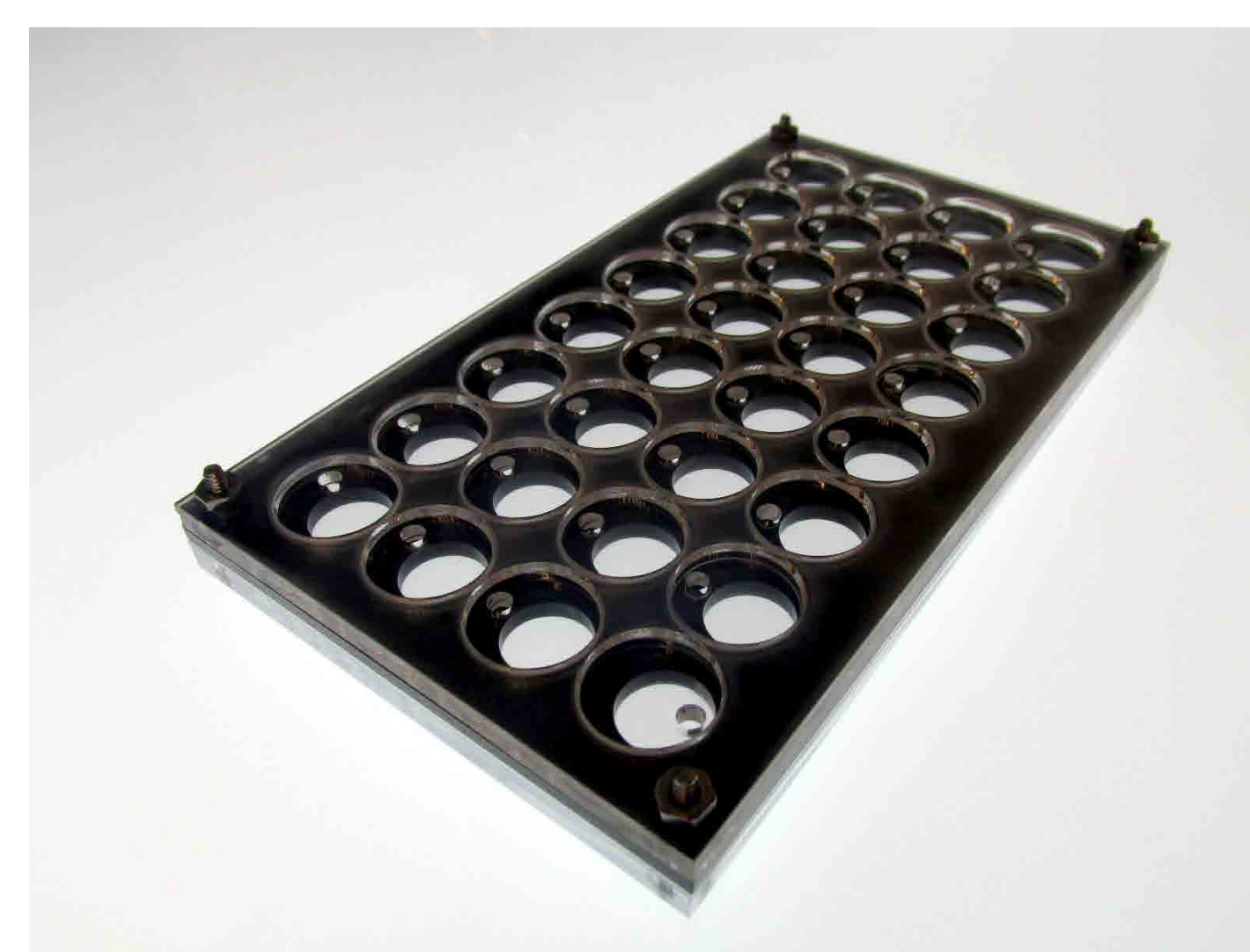
32-chamber arena for fruit fly behavior.
